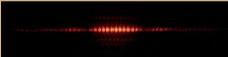
**Figure 2:** *A single-slit (non-interference) pattern.*
